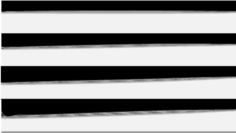
Figure 3. Dynamics of erosion of the interface between the low-solids and high-solids areas for a geometry with the channel inclination angle of 1.5^\circ
