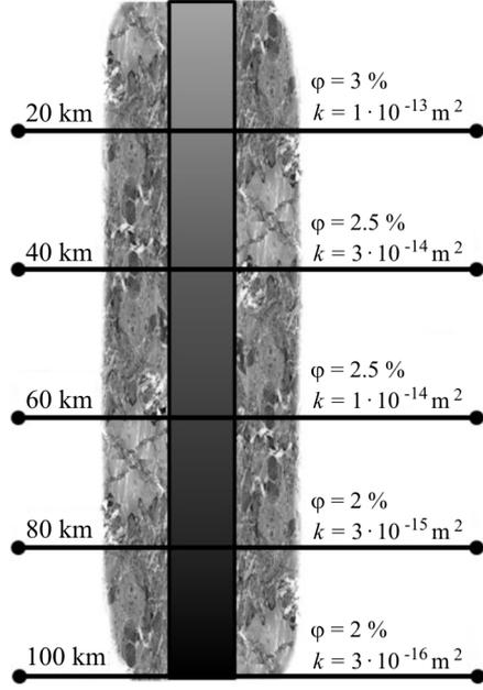
**Figure 1.** The scheme of the permeable zone structure
