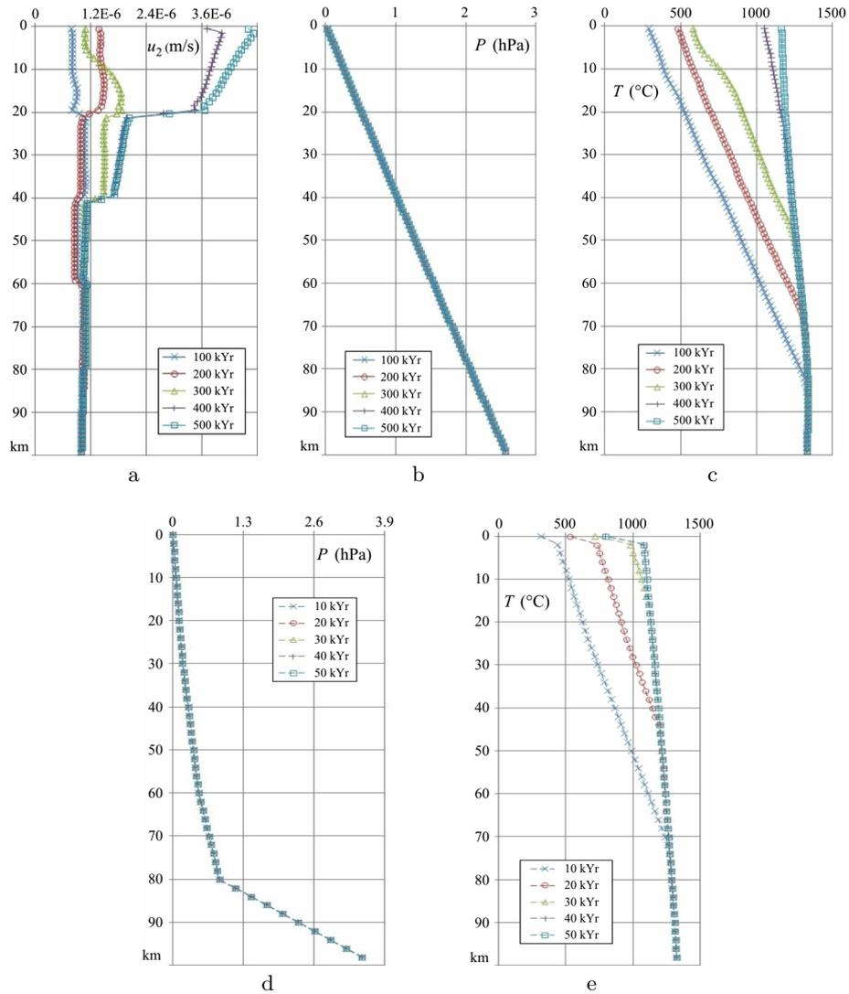
**Figure 2.** The time evolution of the resulting parameters of the filtration flow of the lithospheric fluid in the permeable zone along the Central vertical section of the calculation domain with the non-equilibrium pressure model of compressible two-phase media: a) the vertical components of the velocity vector of the liquid phase, b) pressure, and c) temperature; in the one-velocity Darcy's approximation of d) pressure and e) temperature
