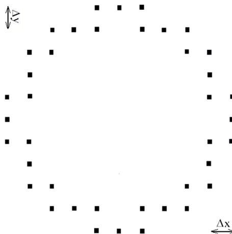
**Figure 1.** The location of the rectangular grid nodes representing the initial circular wave front. The length of the spatial steps along the abscissa and the ordinate axes are  $\Delta x$  and  $\Delta y$ , respectively
