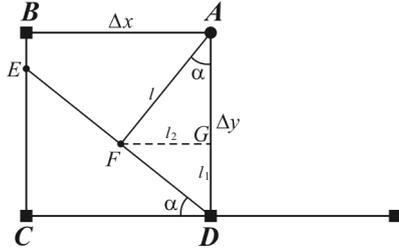
**Figure 3.** The scheme for calculating the arrival time at the point  $A$  based on the known arrival times of the wave at the points  $B, C$  and  $D$ . At the angles of the cell, depths are given
