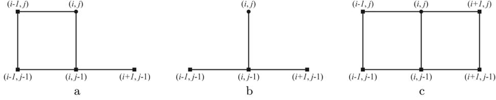
**Figure 2.** The possible configurations for the computation of the wave arrival time to the grid node  $(i, j)$
