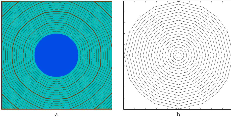
**Figure 6.** The isolines of the calculated wave arrival times from a round source to the nodes of the calculation grid when using the method proposed (a) and as a result of the calculation using the algorithm based on the Huygens principle (b)
