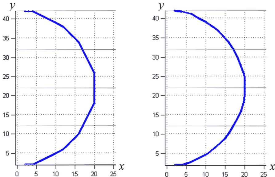
**Figure 7.** Comparison of the wave ray shapes above parabolic bottom before (left) and after optimization (right)
