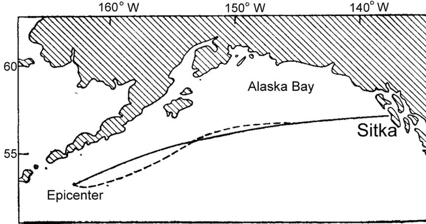
**Figure 1.** The wave-ray route (dashed line) connecting the tsunami source situated near Aleutian Islands and the Sitka Island built by method of variations [1]. The black line presents the geodetic trace being the shortest route on the spherical Globe
