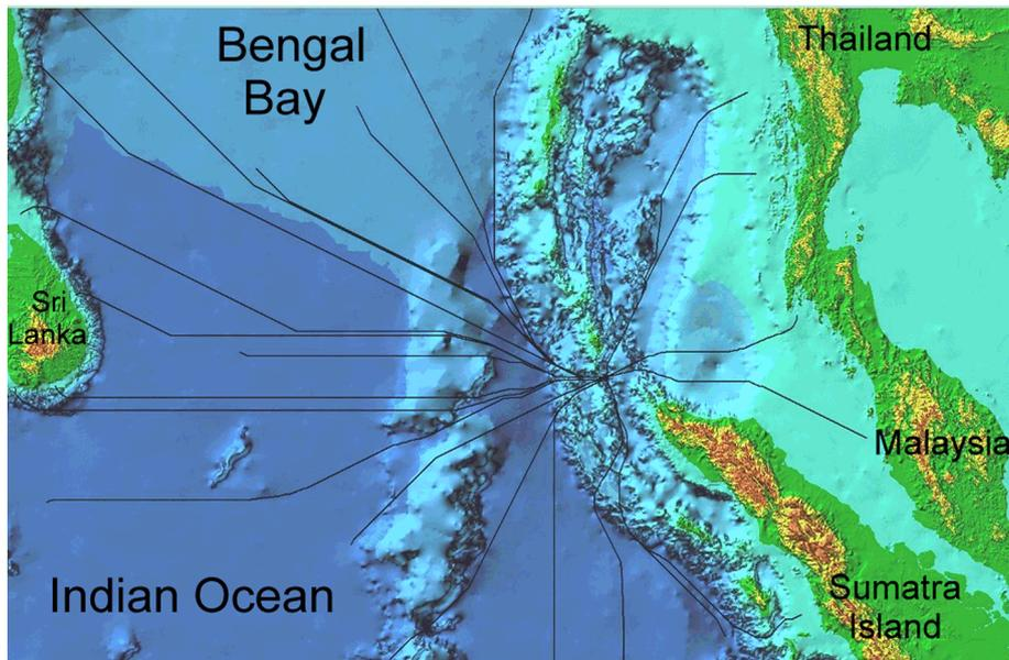
**Figure 5.** The bottom relief and tsunami wave rays in the Eastern Indian Ocean
