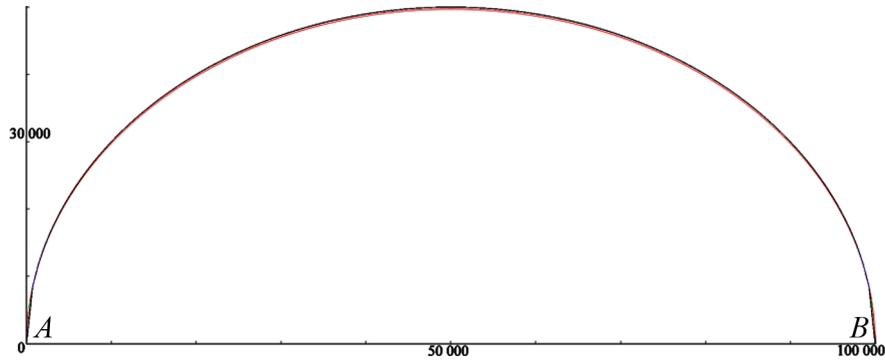
**Figure 4.** A comparison of the exact solution (painted black) with the wave ray constructed by the variation method (painted red) above the parabolic bottom topography
