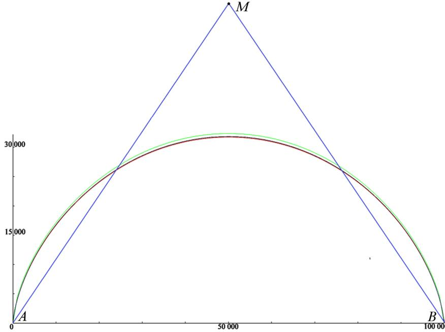
**Figure 2.** Comparison of exact solution with the wave-ray routes obtained by the method of variation: red — the final ray initiated by the straight segment  $AB$ ; black — the exact solution (a segment of the cycloid); and green — the final wave ray trajectory initiated by the broken line  $AMB$
