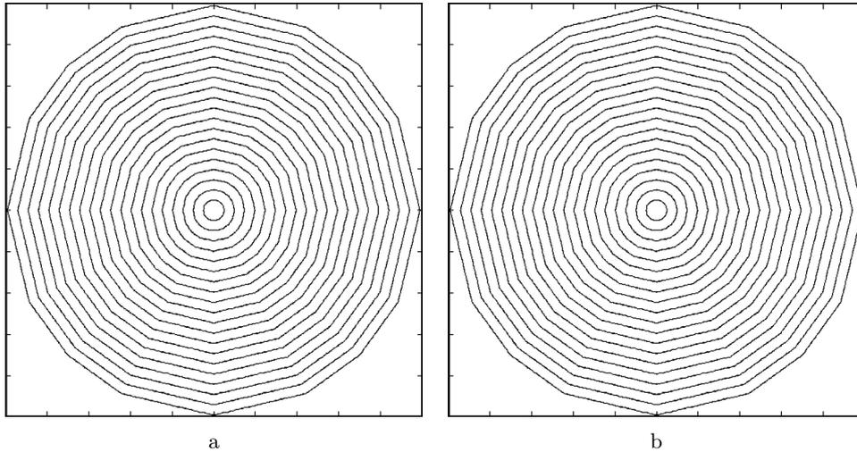
**Figure 9.** A tsunami isochrones as a result of testing the kinematic method for gridded data in the area of the uniform depth. The results of non-optimized method (a) and optimized one (b)
