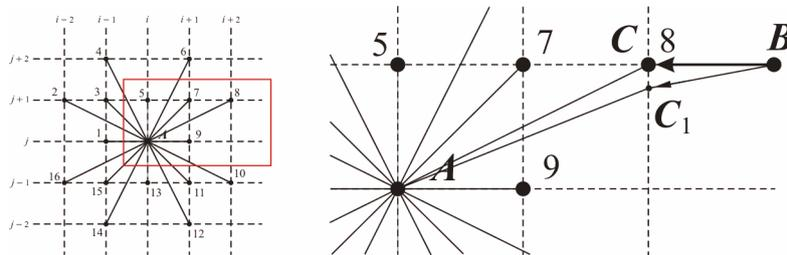
**Figure 8.** A scheme of the travel-time correction algorithm
