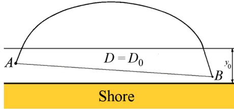
**Figure 3.** A non-unique solution of the edge problem for the wave ray in the case of the shelf of constant depth
