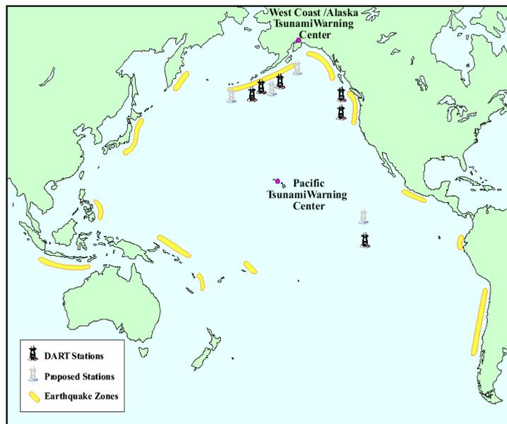
Figure 5. Location of installed (dark icons) and planned (light icons) DART stations
