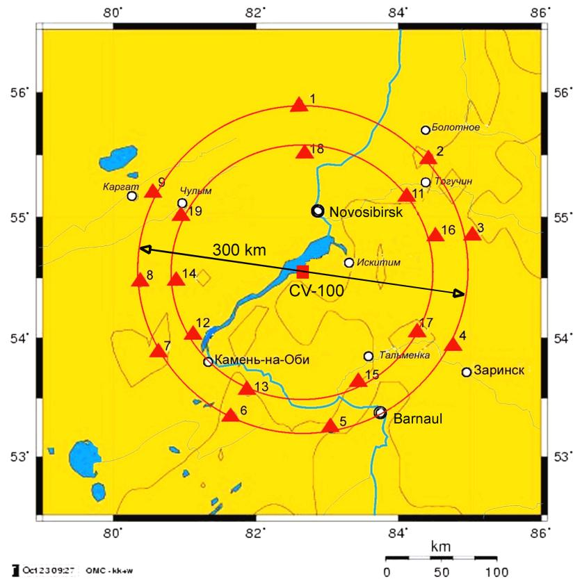
**Figure 7.** The scheme of experiment “Circle”
