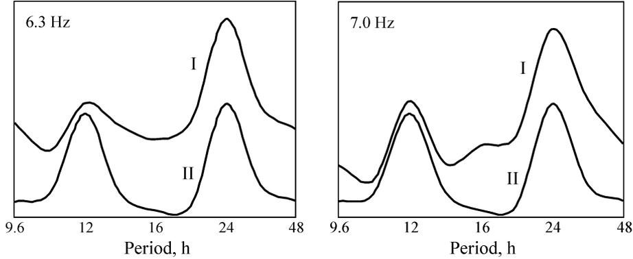
**Figure 6.** An average spectra of variations of vibrosignal parameters (I) and tidal variations of gravity (II). Vibrator CV-100, frequencies 6.3, 7.0 Hz, distance 356 km
