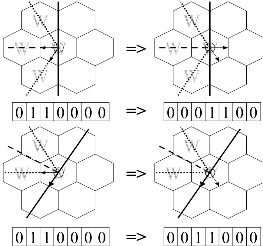
**Figure 6.** Reflections from the wall cell (smooth wall)
