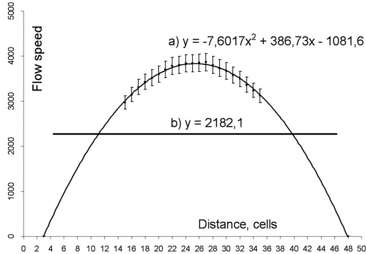
**Figure 7.** Dependence the flow speed from the distance to the wall
