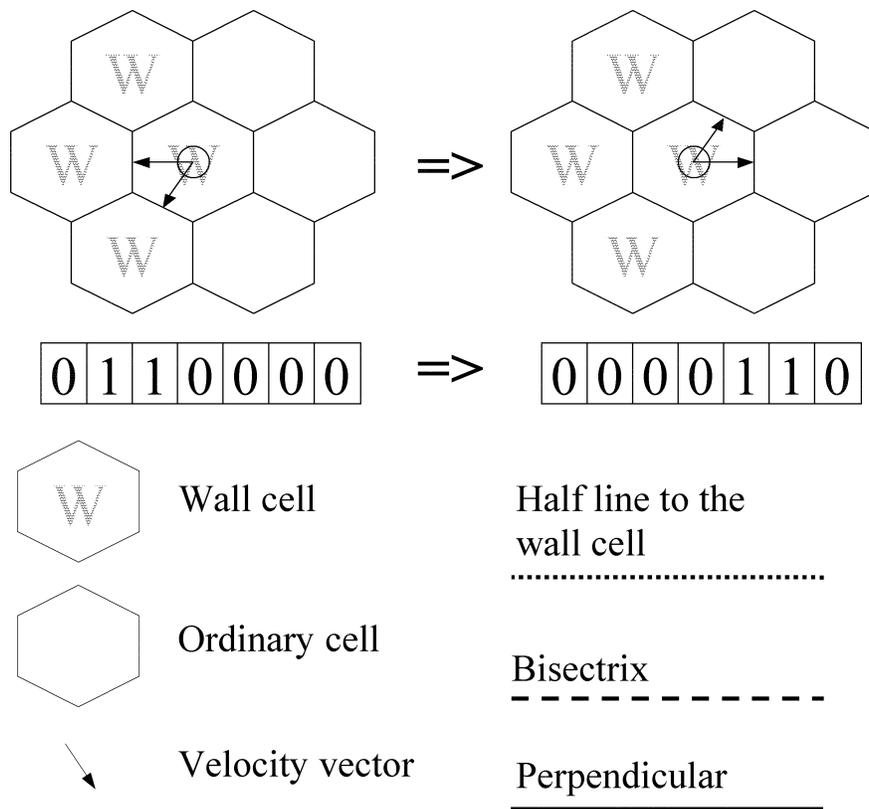
Figure 5. Reflections from the wall cell (wall with friction)
