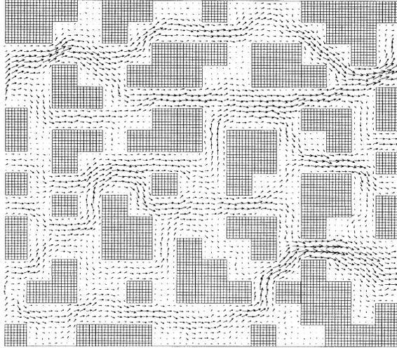
**Figure 4.** The speed field of the 2D flow (from [5])
