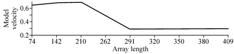
**Figure 12.** A change in the model wave velocity in aluminium-ebonite medium
