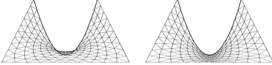
**Figure 1.** Grids in a concave domain generated by the solution to equations (9) (left) and by the solution to equations (5) (right); both with respect to the Euclidian metric
