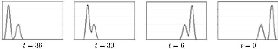
Figure 3. Unidirectional composition of two CA: a totalistic parity CA simulating a soliton-like process and an averaging CA for transforming the CA results to a comprehensive form. Three snapshots of the composed CA are shown for t = 6, 30 and 36
