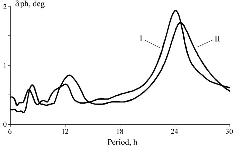
**Figure 5.** The average spectra of variations of vibrosignal parameters (I) and tidal variations of gravity (II). Vibrator CV-100, frequency 6.75 Hz, distance 430 km
